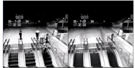
Fig. 3: Screenshot: Left frame is from original video; right frame is the background after applying IALM algorithm
