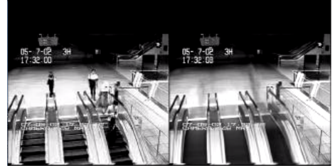
Fig. 2: Screenshot: Left frame is of original video; right frame is the background after applying Alternate Projection algorithm
