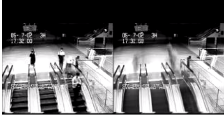
Fig. 5: Screenshot: Left frame is of original video; right frame is the background after applying Fast gradient based method
