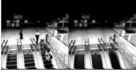
Fig. 4: Screenshot: Left frame is of original video; right frame is the background after applying Fast gradient based method
